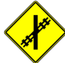
RAILWAY CROSSING ANGLED WA-18L/R 750mm x 750mm
