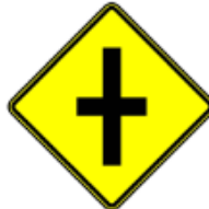
CONCEALED INTERSECTION WA-11 600mm x 600mm
