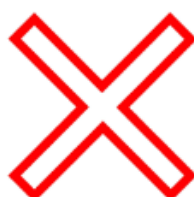
CROSS BUCK RA 6 CROSS LENGTHS 1200 x 200mm
