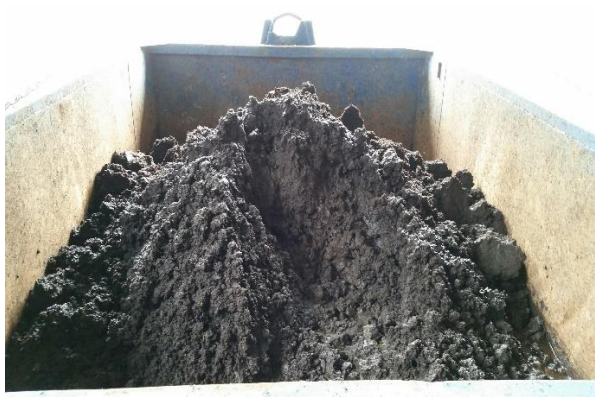
Dewatered sludge (dirt removed from water by centrifuge) ready for disposal
